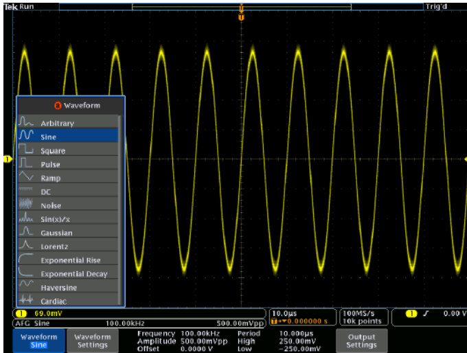
Waveform type selection in the integrated AFG.
